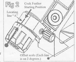
(Fig 2 "A") are aliened (fig 2). If you can not get them to align properly, then rotate the dial to the next set of lines and repeat this process. After you have completed this, lock down the fletching plate adjustment knob (Fig 1 "F"). This step is not necessary for a 4 X 90 Fletching.
